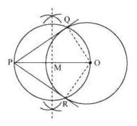
$\angle$ PQO is an angle in the semi-circle. We know that angle in a semi-circle is a right angle.  $\therefore \angle$  PQO = 90°  $\Rightarrow$  OQ $\perp$ PQ
