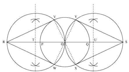
$\angle$ RVO is an angle in the semi-circle. We know that angle in a semi-circle is a right angle.  $\therefore \angle$  RVO = 90°  $\Rightarrow$  OV $\perp$ RV
